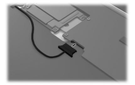
2. Disconnect the WLAN antenna cables (1) from the terminals on the WLAN module.
